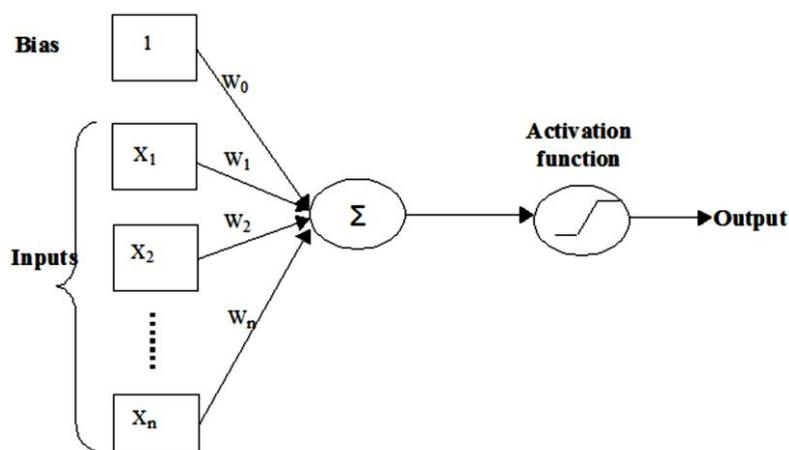
**Figure 2:** The figure presents the simple Neural Network Model.
