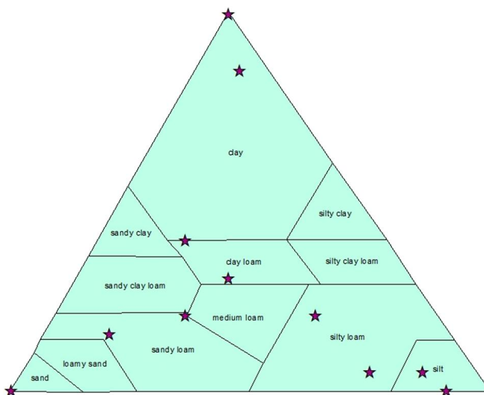
Figure 2: The figure presents the points distributed on the soil triangle using the SOIL TRIANGLE TOOL software tool.
